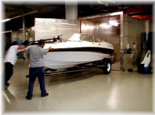
Photo 5. Vehicle Insertion Into the SHED
