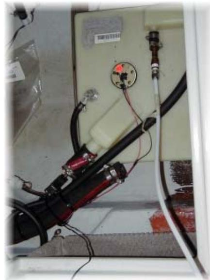
Photo 4. Instrumented Fuel Tank
