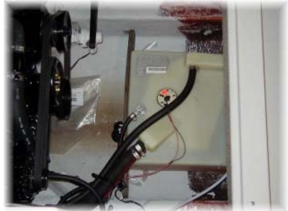
Photo 3. Production Fuel Tank and Lines
