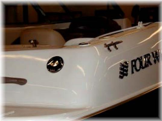
Photo 2. Fuel fill – starboard, aft (right, rear)
