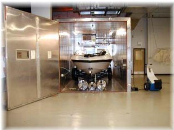
Photo 6. Boat in SHED, Circulation Fans in Position
